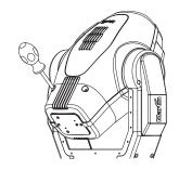
Convenient 1/2 turn screws make for easy component accessibility and simple lamp adjustments.
