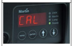
A 4-digit LED readout allows the user to customize settings for easy programming. Error messages are easily understood, lamp and fixture usage is displayed and the readout flips for easy reading in any position.
